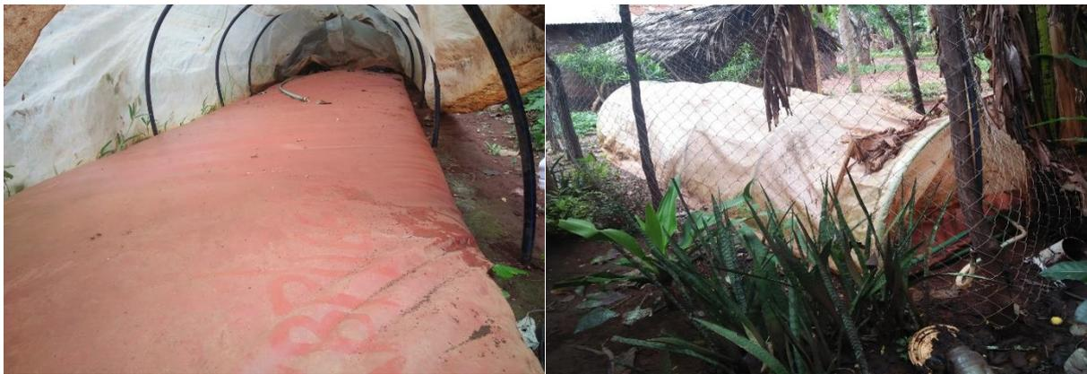
Figure 17(a) Flexi Biogas Showing Digester Envelop. (b) Covered by Micro-Greenhouse Tunnel
